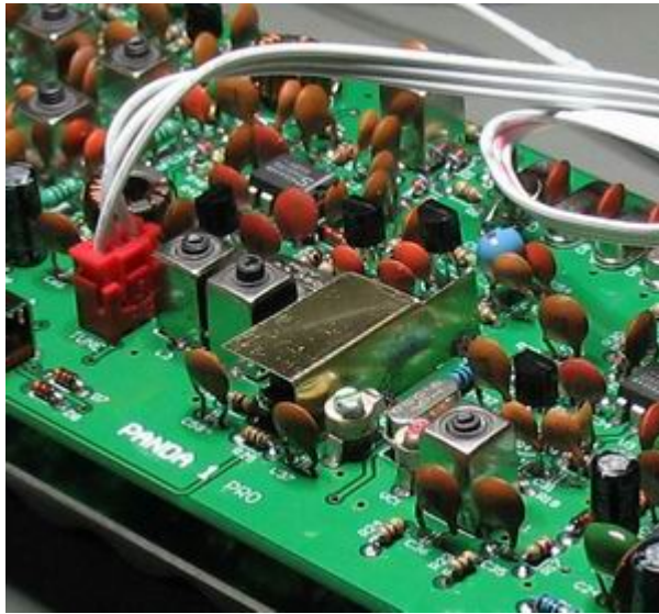
Fig.5 If a larger piece of tin strip is at hand, more perfect screen could be made, shielding RL1.
