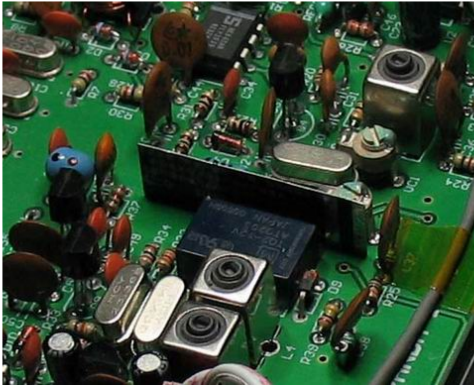
Fig. 3 Place the metal strip in such a place as to separate VC2 from RL1.
